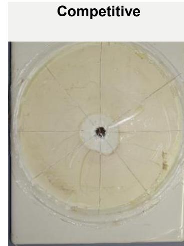
Loss of adhesion 2-3mm
