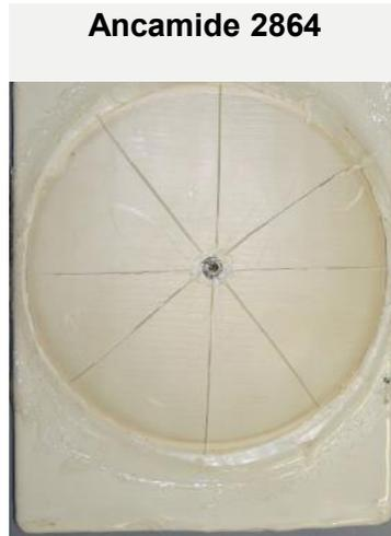
Loss of adhesion 1mm
