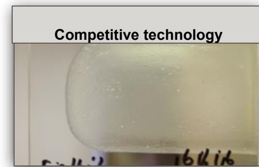
Both panels applied and cured at 5°C and 60% relative humidity
