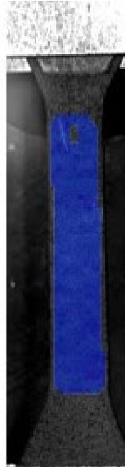
Use of high speed camera and digital image correlation to post process true strain rate
