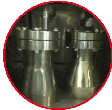
PCT Hydrolysis Tester
