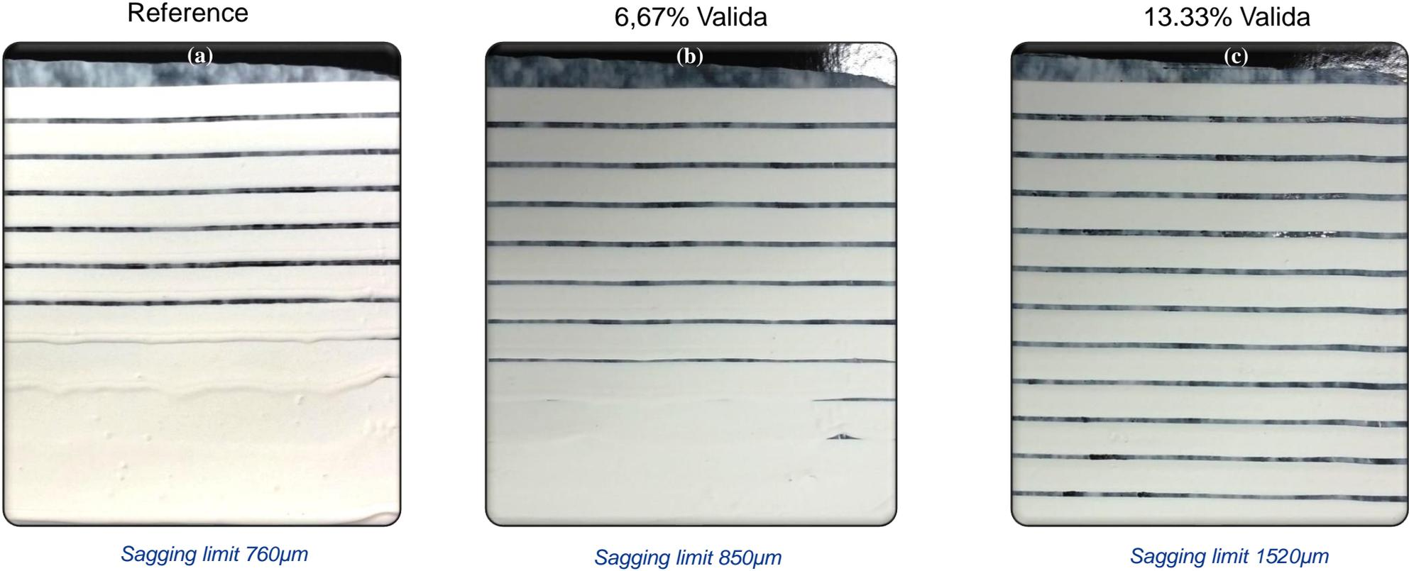
**Figure 1:** (a) Reference, (b) 6.7% Valida gel, (c) 13.33% Valida gel
