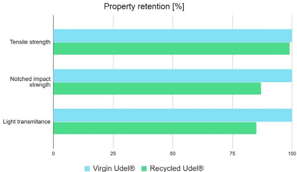
Recycled Udel® PSU maintains excellent properties, while allowing a significant decrease of environmental impact
