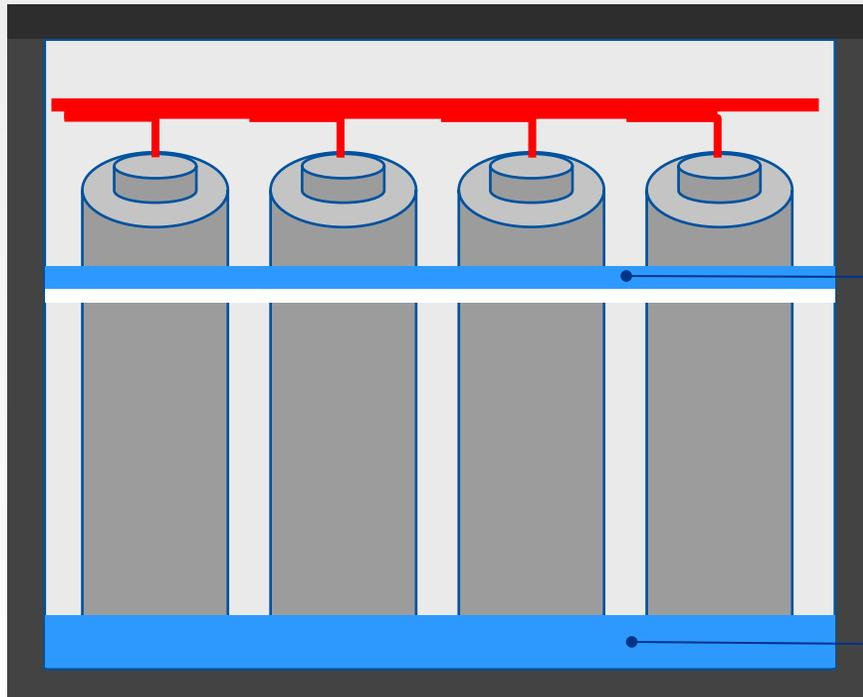
Thermal interface material adhesive or sealant,
