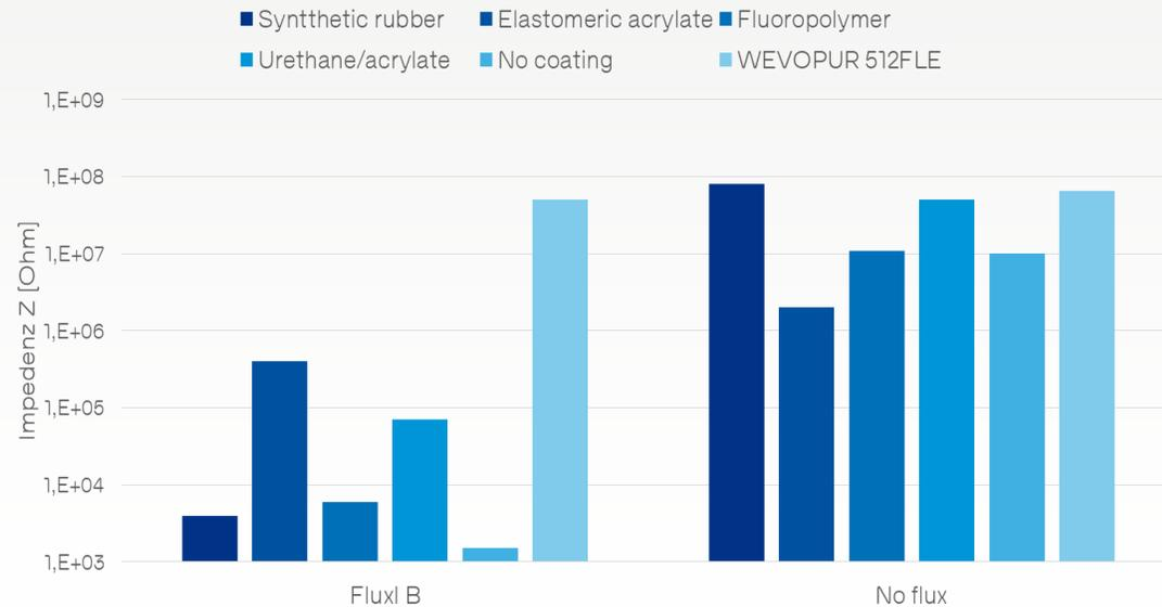
Comparison of the behaviour of WEVOPUR 512FLE with standard conformal coatings
