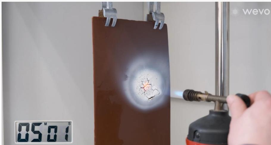
>1000 °C flame on a 1mm silicone coated steel plate
