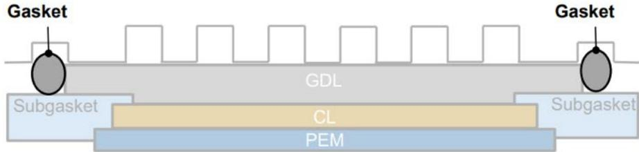
The diagram shows a cross-section of a fuel cell assembly. From top to bottom, the layers are: Gasket (top), Subgasket, GDL (Gas Diffusion Layer), CL (Catalytic Layer), and PEM (Proton Exchange Membrane). The Gasket and Subgasket are shown as blue blocks with circular features. The GDL is a grey layer with a grid pattern. The CL is a yellow layer, and the PEM is a blue layer. The Gasket and Subgasket are positioned on either side of the GDL, CL, and PEM layers.
