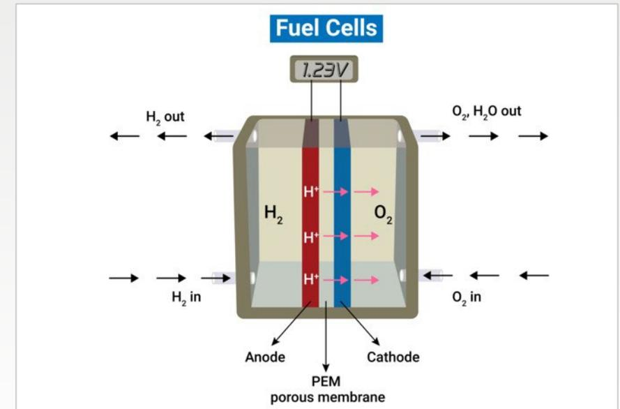
The most important type of fuel cell for many applications today is the proton exchange membrane fuel cell (PEMFC). Such a fuel cell usually uses hydrogen as fuel. This is generated either by steam reforming from methanol or methane and in the future from renewable energy by electrolysis (green hydrogen).
