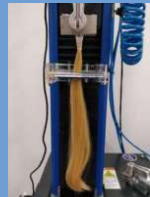
Instron 23-2S test device with comb holder
